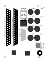
The **AMG4708EG** is a rackmount data receive unit designed to transmit and receive up to 16 data or audio signals plus full duplex 100BaseT Ethernet connectivity over two singlemode fibres. The 16 data/audio channel interfaces, whether RS232, RS422, RS485, 20mA, TTL, Contact Closure, Lonworks or Audio, are defined at manufacture by the addition of daughter boards fitted onto the Data Expansion Board Boards A and B.
